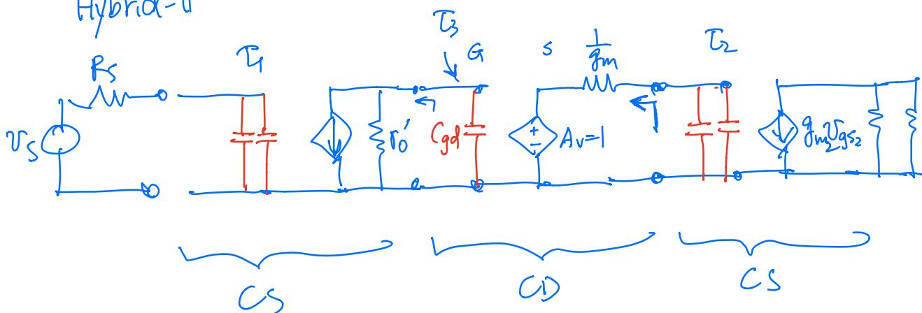
$$A_V = A_{V1} A_{V2} A_{V3} \frac{R_L}{R_{out} + R_L} \quad \text{same}$$
