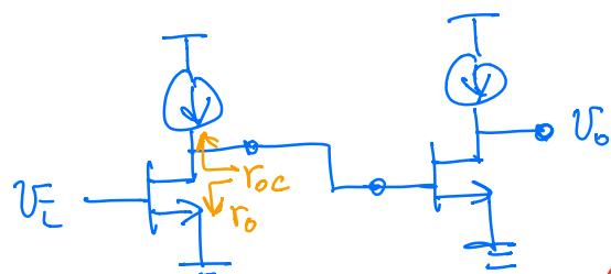
$$A_V = \left( \frac{R_{in}}{R_s + R_{in}} \right) \cdot A_{V1} \cdot \left( \frac{R_{in2}}{R_{out1} + R_{in2}} \right) \cdot A_{V2} \cdot \left( \frac{R_L}{R_{out2} + R_L} \right)$$
